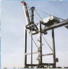
RMQC - Container crane, Penn Terminals, Philadelphia, USA 40,7 t x (41,8 + 18,288 + 18,3) m
